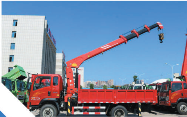
随车吊 Truck Mounted Crane
