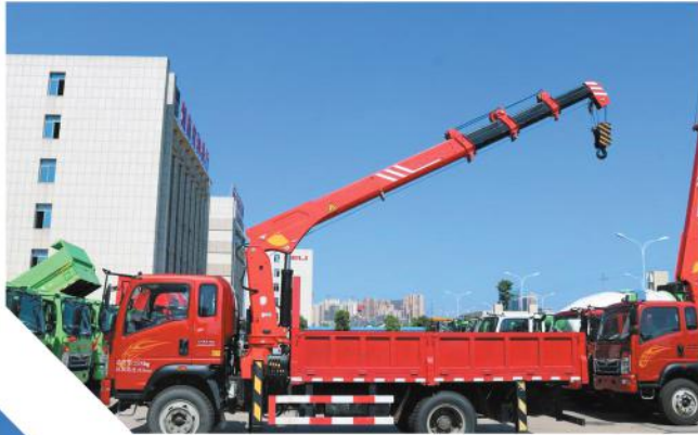
随车吊 Truck Mounted Crane
